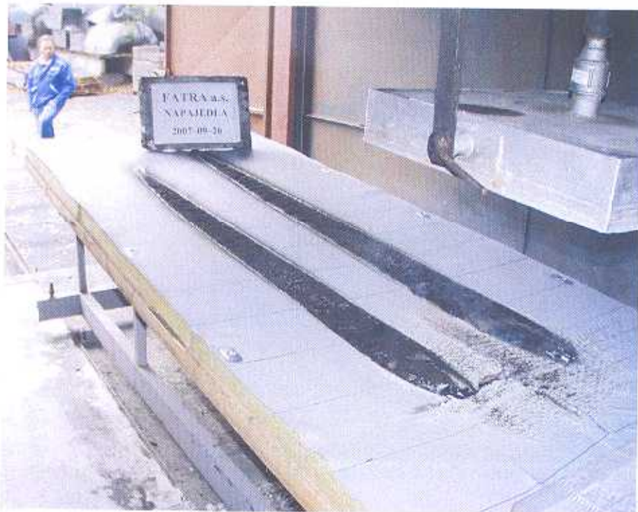
Photograph no. 2 - Test specimen I (gradient 5°) after termination of the test
