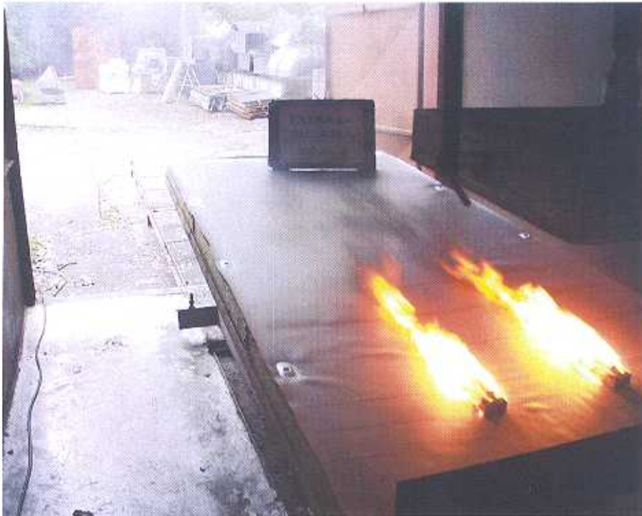
Photograph no. 3 - Test specimen II (gradient 5°) after the start of the test
