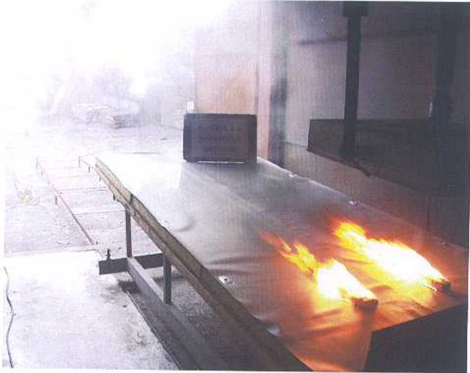
Photograph no. 1 - Test specimen I (gradient 5°) after the start of the test
